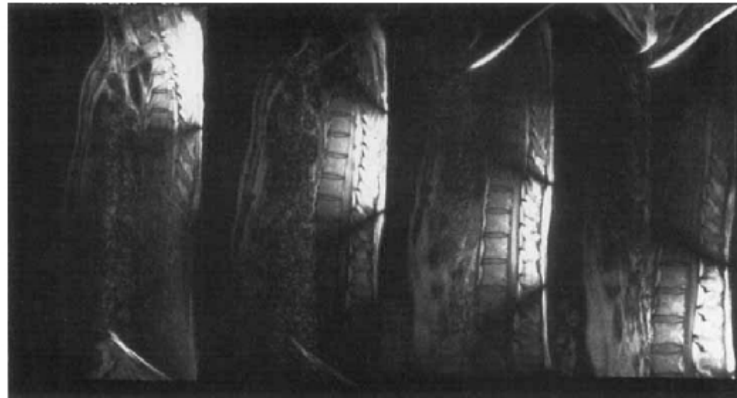
FIG. 16. Four sagittal images taken with the spine array shown in Fig. 13. Although all four coils are simultaneously receiving data, there is no sign of coupling between coils. FOV = 48 cm, 512 × 512 pixels, NEX = 2, 5 mm slice, T_R = 400 ms, T_E = 20 ms, imaging time = 6:50, B = 1.5 T. Phase encoding is in the y direction. Only the central 256 points in the horizontal direction are shown. Artifacts at the top and bottom of the images are due to wraparound.
